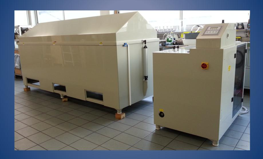
Chamber for continuous salt spray and condensation test and cyclic tests.
